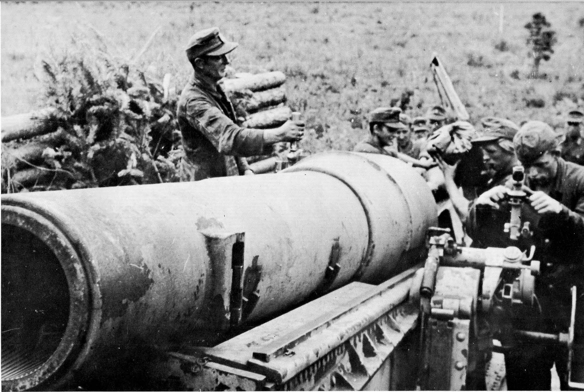
As mentioned on the preceding page, the cartridge is then loaded. The breechblock is then immediately closed by the K 2 (breech mechanism handler) so that the mortar can be reported as "ready to fire."
