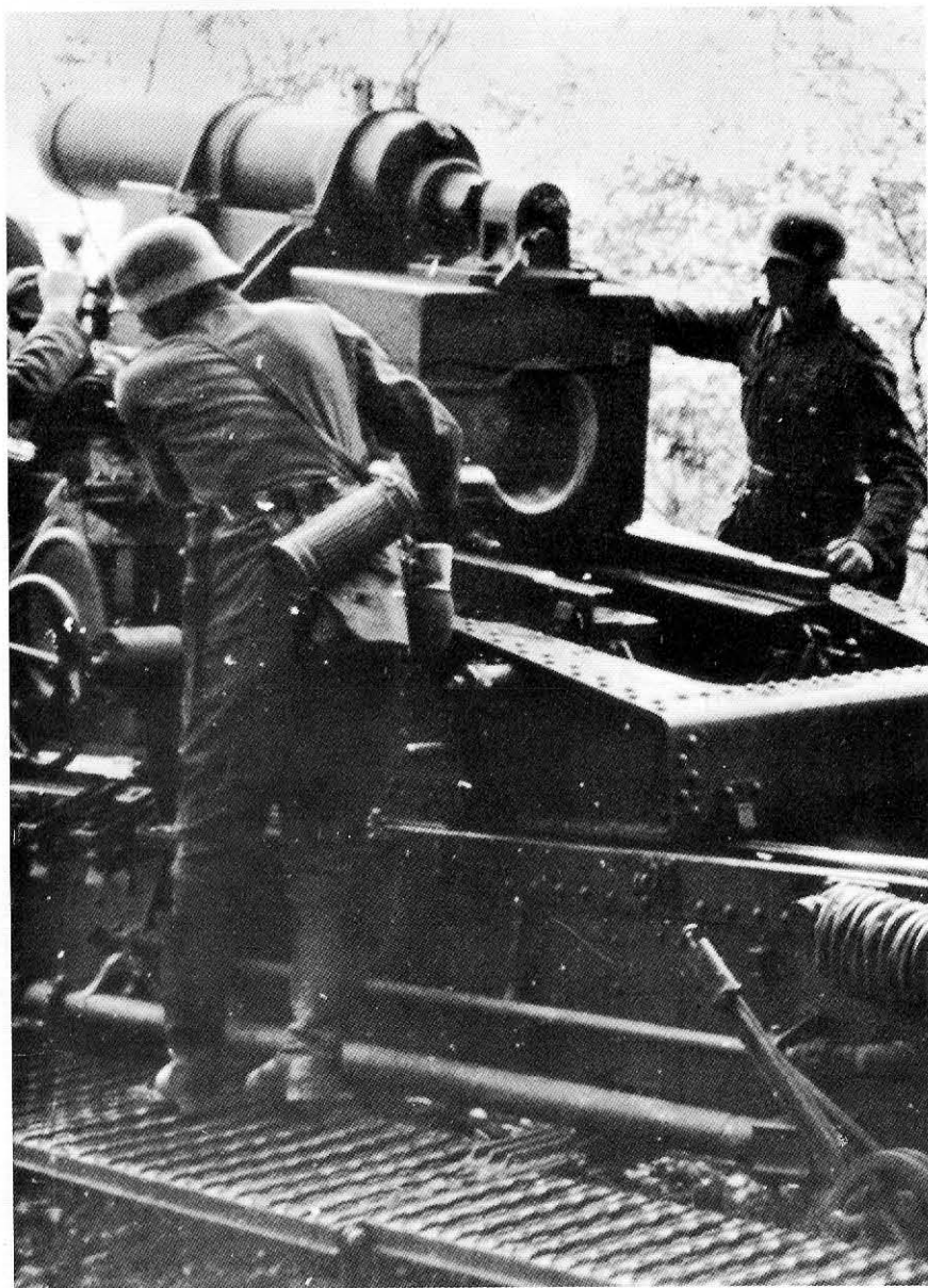
After loading, the barrel is brought to the proper elevation. There are two barrel elevating drives, one for quick, rough adjustments and the other for slower, finer adjustments.
