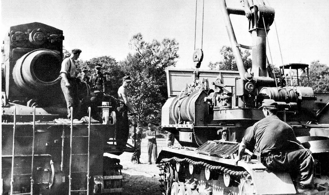
Above: The Mun.Pz.IV uses its winch to offload a 2.117 ton concrete piercing shell, which can penetrate 2.5 meters of concrete or 4 meters of armor plating.
