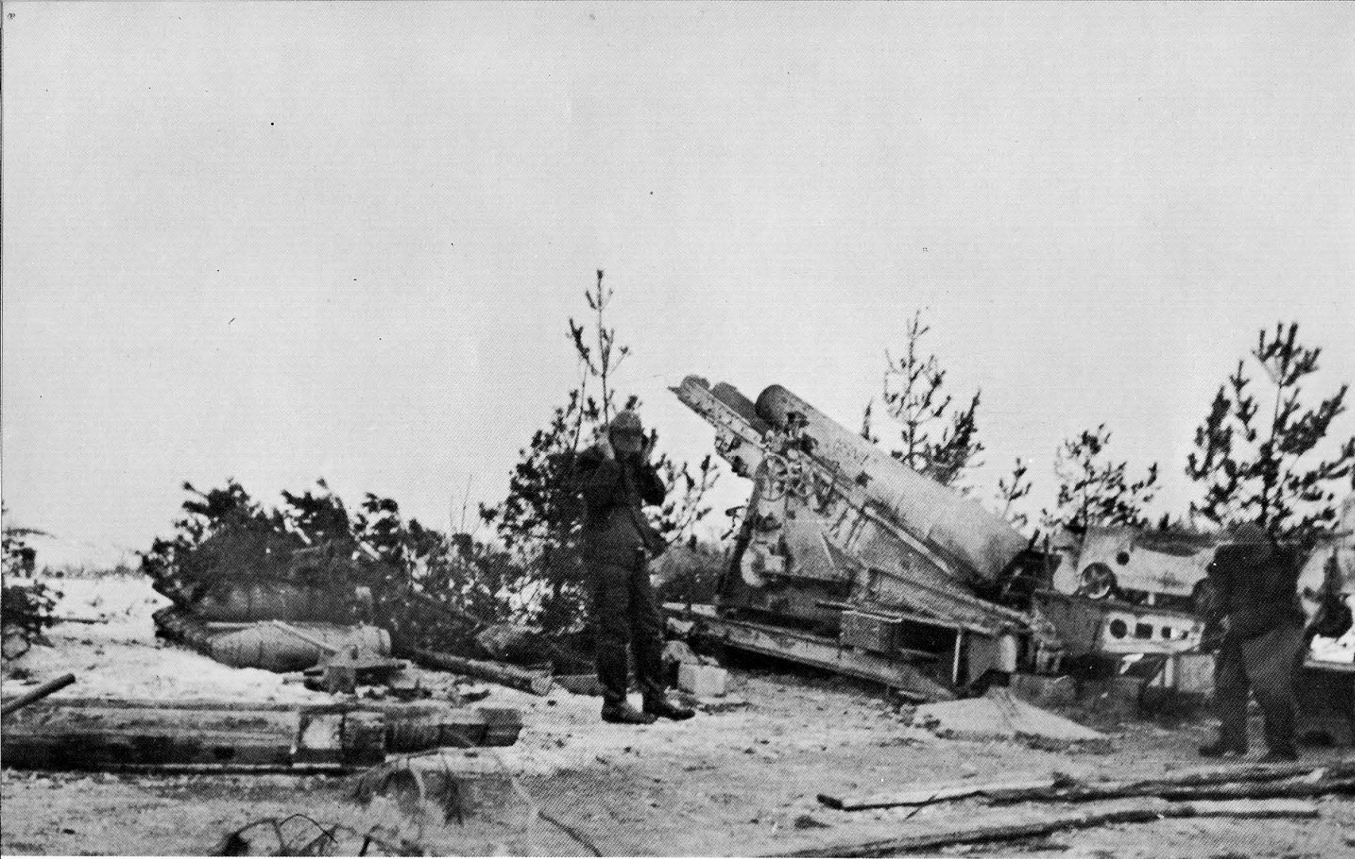
Russia, winter of 1943/4 the barrel of a 28 cm Mörser (f) M 16 recoils after firing. Note that the elevation is at the lower end of the upper elevation group. A pile of shells lies ready to be fired.
