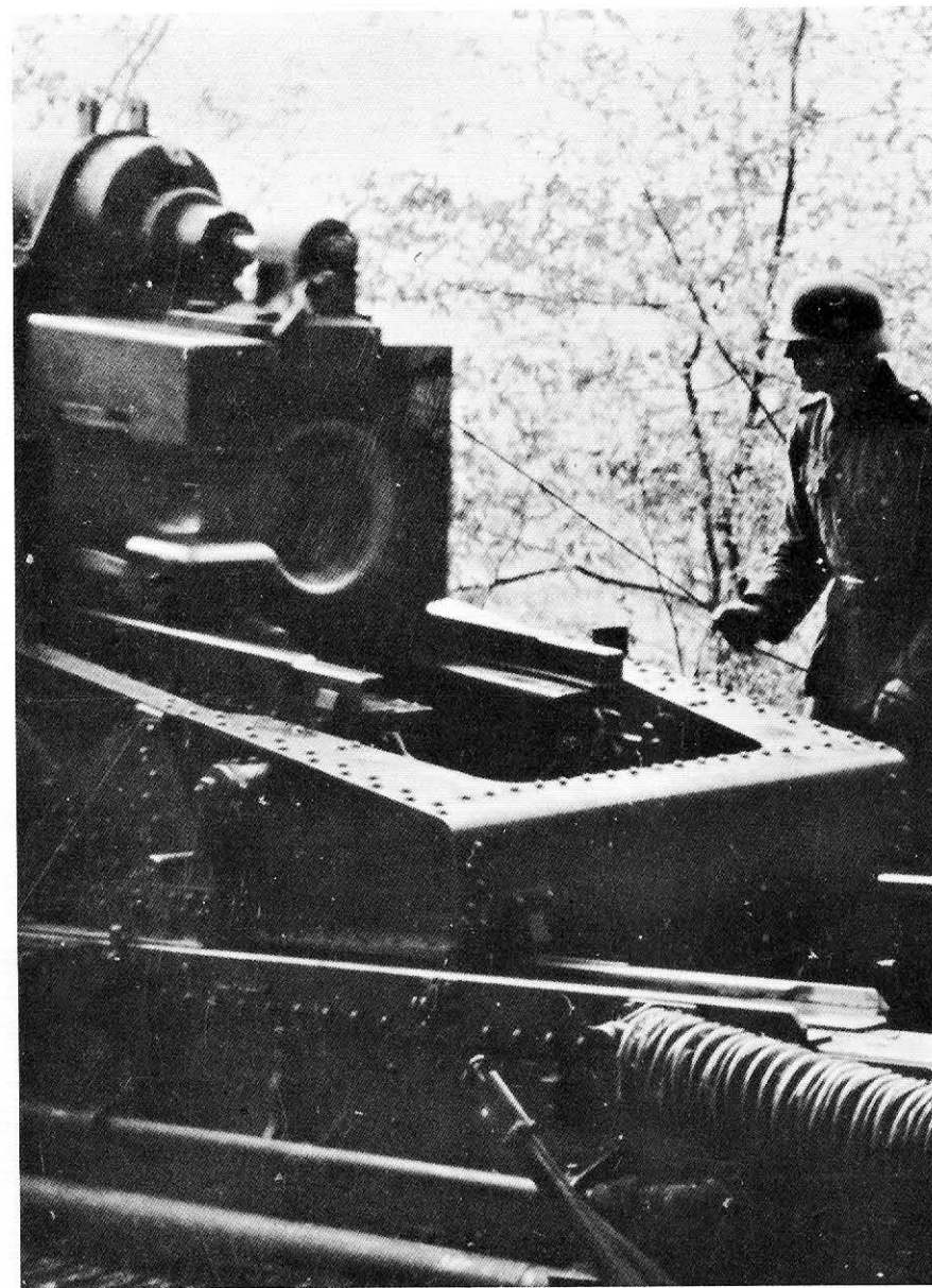
The K 2 (breech mechanism handler) pulls the lanyard to the firing mechanism taut, awaiting the command to fire.
